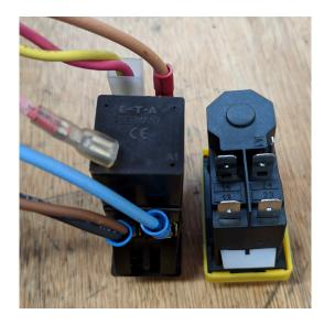
**Step 3:** Remove the Brown wire from Terminal (22) and place it firmly on Terminal (14) of the new switch.
